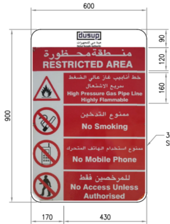
SIGNBOARD (FRONTSIDE) SCALE=1:10
