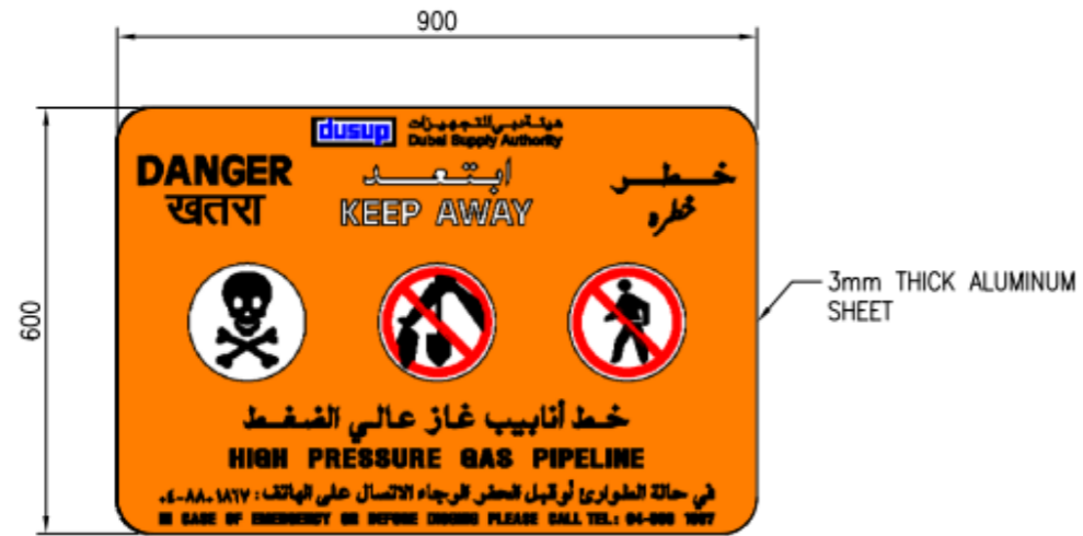
SIGNBOARD (FRONTSIDE) SCALE=1:10
